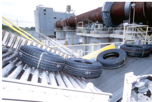
At the Atlanta cement plant, USA, scrap tires are used as an alternative fuel. They are placed whole in the kiln.
