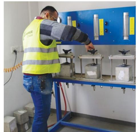
Testing water penetration - central lab Erbil
