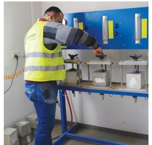
Testing water penetration - central lab Erbil
