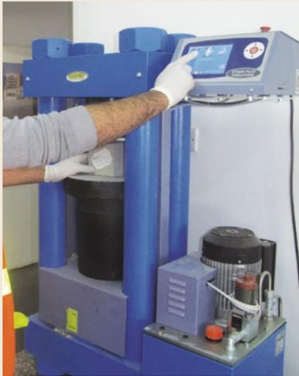
Concrete cubes compression testing
