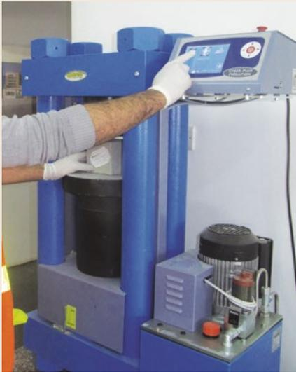
Concrete cubes compression testing
